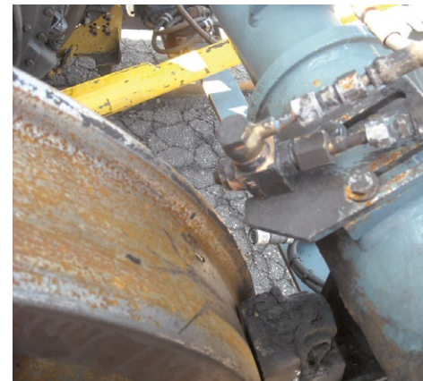
▼ The ejectors must be positioned as close as possible to the wheel-rail contact
