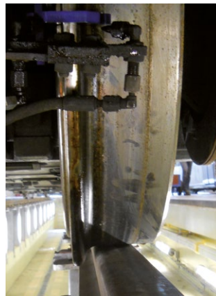
▼ The ejectors must be positioned as close as possible to the wheel-rail contact
