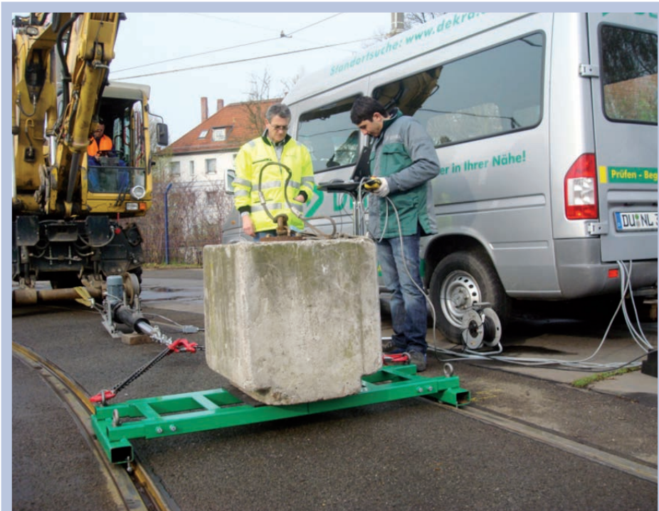
Fig. 2: Measurements of the friction coefficient (parts of rubber tyres were used as the friction partner on the rail head)
